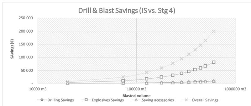
**Figure 10. Drill and Blast Savings**
