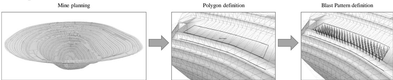
Figure 3. Blast design process
