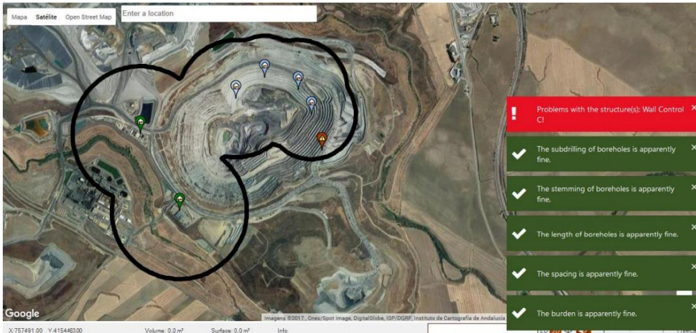
Fig. 396 – Detection of problems with the structures.
