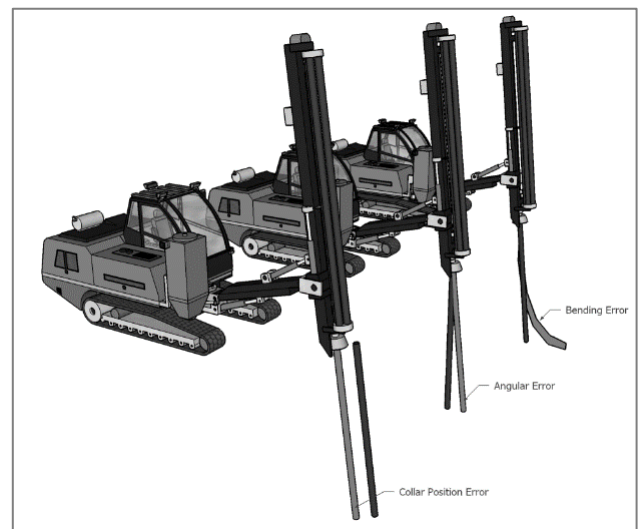
Figure 2 - Typical drilling errors
