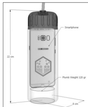
**Figure 3. Smartphone used to measure holes**
