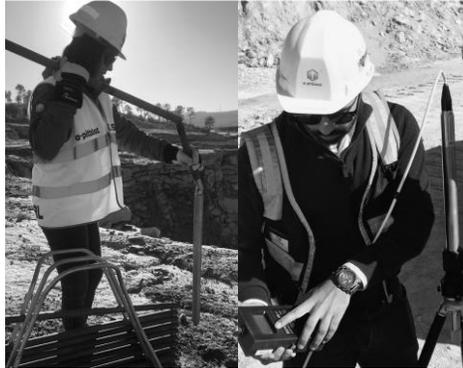
**Figure 2. Rodded Boretrak (left) and Cable Boretrak (right)**
