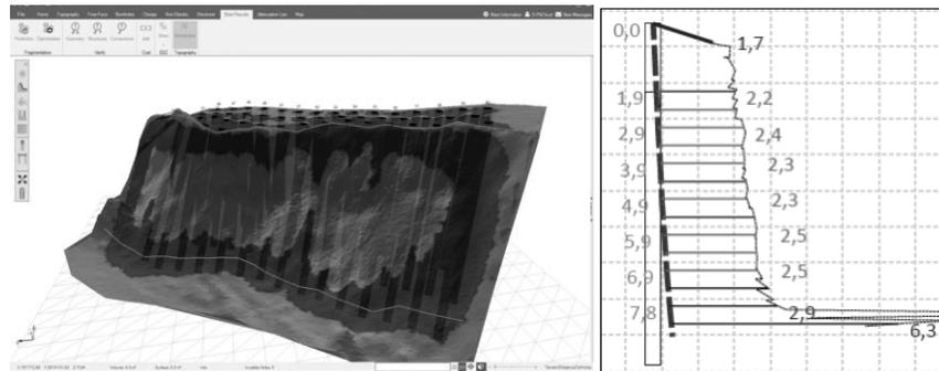
**Figure 4. Critical Burden Detection (O-Pitblast)**
