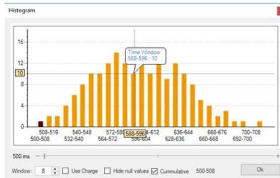
Figure 312 - Histogram - Number of Holes per Delay.
