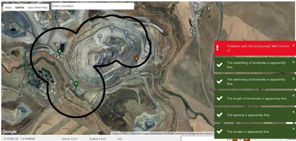
Figure 434 - Detection of problems with the structures.
